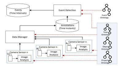
**Figure 2.** Block diagram of the prototype system. Sensors (here IP-based surveillance cameras with their companion image analyzers) annotate observations with the help of vocabulary provided by *Time, Property*, and *Object* ontologies, and leave annotations in sub part of the data model. The Data Manager checks data aggregation and assigns confidence measures to annotations. Event Detection mines events from annotated observations.
