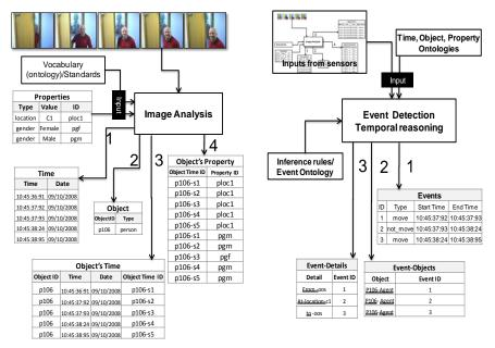
**Figure 3.** Schematic data flow. The left-hand side shows the order of asserting a sensor's observations (e.g. an IP camera with its companion image analyzer) in the data model; event detection is shown on the right-hand side.
